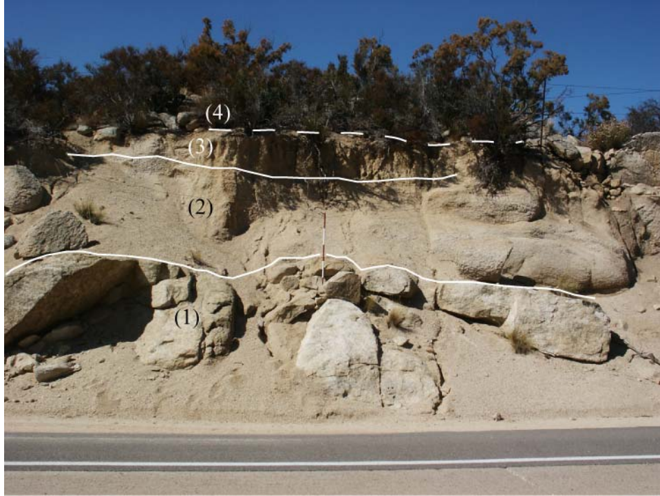
Figure 3. Mollisol profile, Peninsular Ranges, southern California. Note the layers designated (1), (2), (3), and (4). The staff is 5 feet in length.
